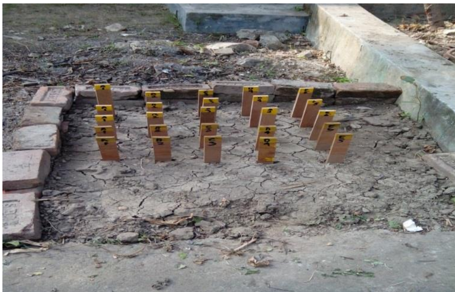
Sample exposed in graveyard test
